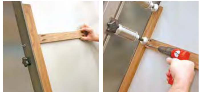
Flush Face Frames Made Easy: 1) Align stile and rail along squaring fence 2) Adjust clamp cylinder and secure joint line 3) Drive self-tapping screw
