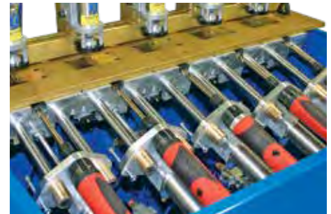
Don't let bit changes slow you down. The simple and straightforward design of the DK5100—and all of our machines—lets you make easy bit changes in 60 seconds or less.
