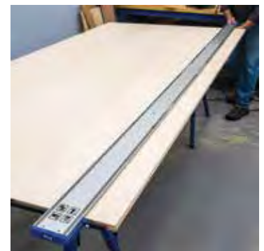
Add 2 feet (61cm) to your Straight Edge Guide to crosscut and rip cut sheet goods
