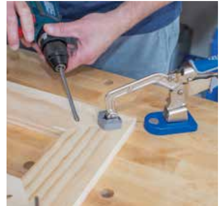
Bench Clamp keeps pieces perfectly aligned to create tight-fitting joints.
