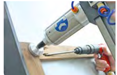
Flush Face Frames Made Easy: 1) Align stile and rail along squaring fence 2) Adjust clamp cylinder and secure joint line 3) Drive self-tapping screw
