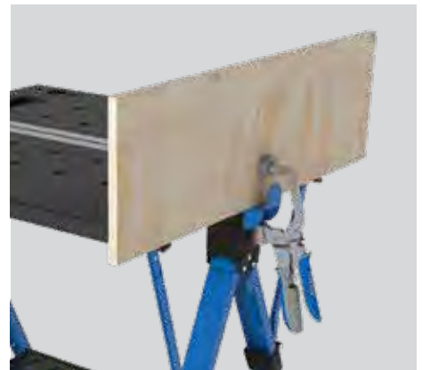
Use the Bench Clamp like a vise to hold objects vertically as you work.
